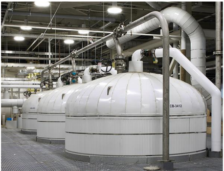
The Sarnia facility uses yeast to produce succinic acid at low pH
